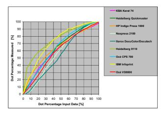
Figure 3. Tone curves of VS 9000 compared to tone curves of other printing engines
