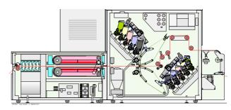
Figure 2. VS 9000 paper input, print module and fusing module
